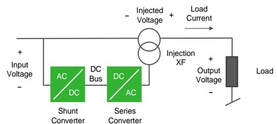
Figure 1: UPFC architecture of an LVR
