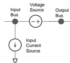
Figure 2: static model of an LVR
