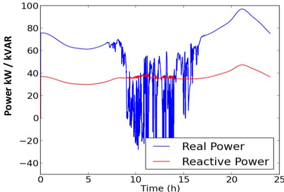
Figure 7: Time-varying power output at feeder source.
