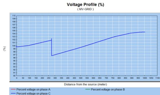
Figure 10: Voltage profile for low load / max PV scenario, from CYMDIST using LTC as an approximation for LVR.
