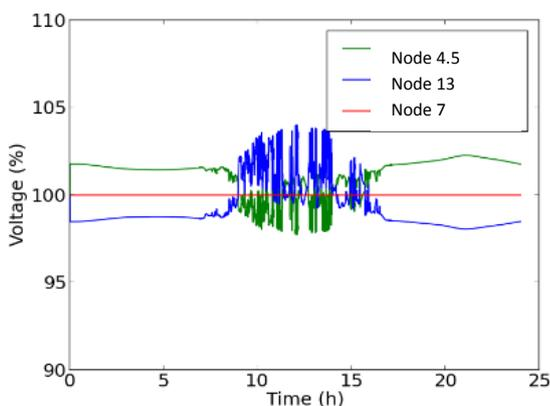
Figure 8: Time-varying voltage at 3 points in the feeder.
