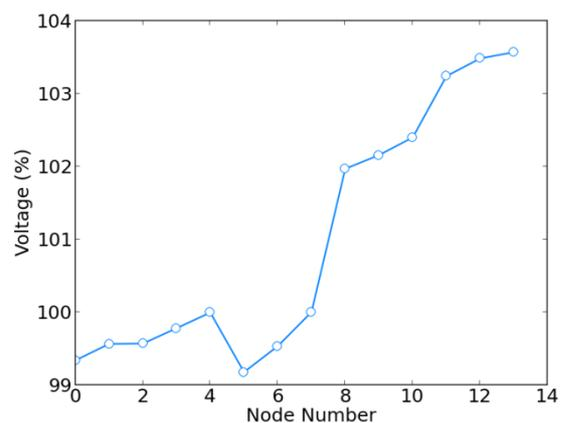
Figure 6: Voltage profile for low load / max PV scenario. Voltage at node 7 is regulated to 100%.
