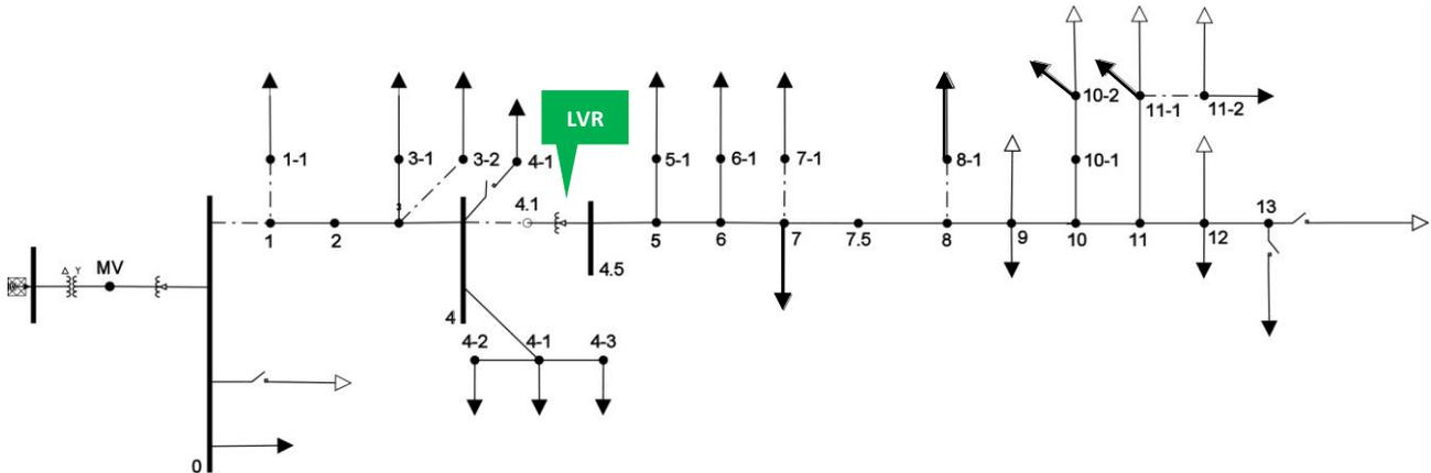
Figure 4: Generic secondary distribution network with LVR located between nodes 4.1 and 4.5. Loads are indicated by black arrows; PV systems are indicated by white arrows.
