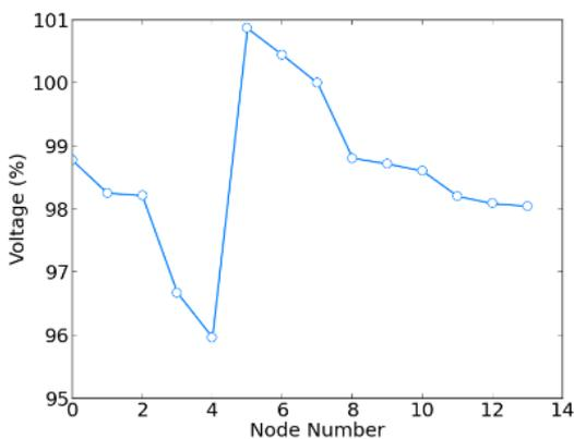
Figure 5: Voltage profile for high load / no PV scenario. Voltage at node 7 is regulated to 100%.
