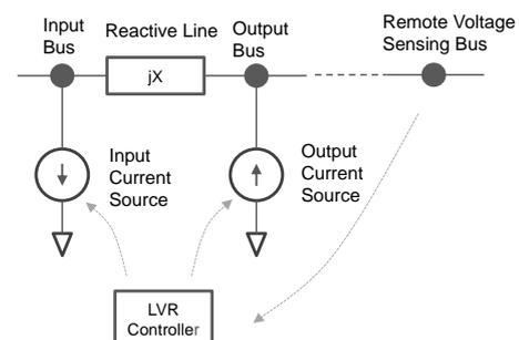
Figure 3: Norton equivalent of the static model
