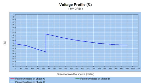
Figure 9: Voltage profile for high load / no PV scenario, from CYMDIST using LTC as an approximation for LVR.
