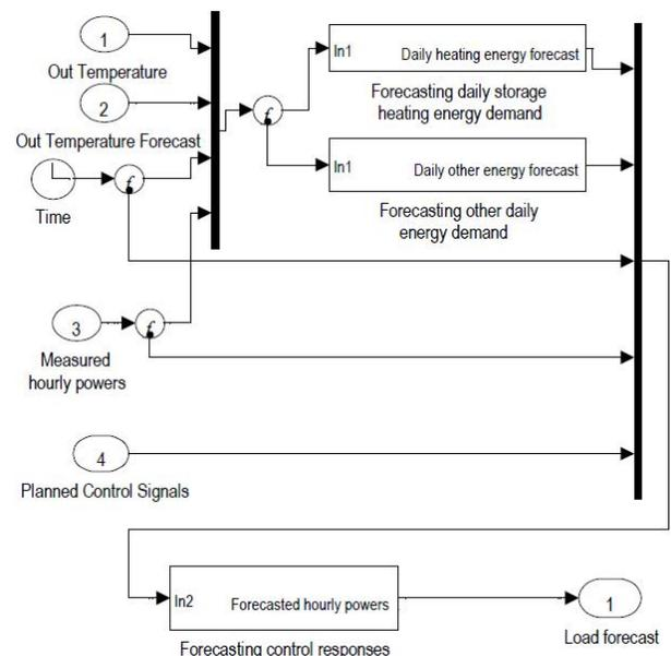
Fig. 1. Simplified overview of the load response forecasting approach
