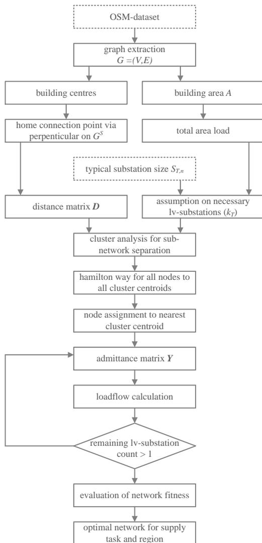
Fig. 1. Flow chart of the network generation process
