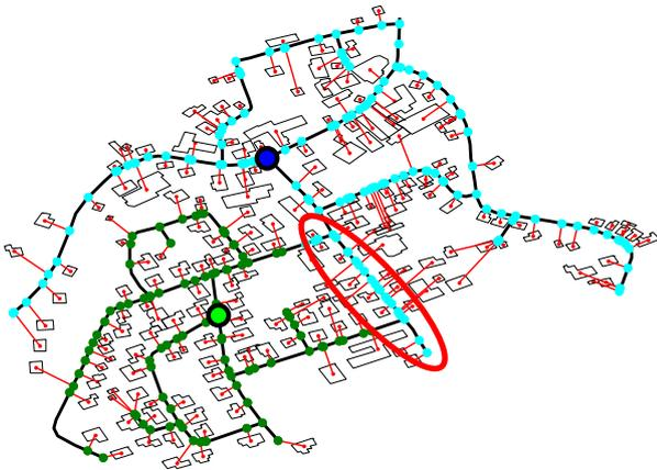
Fig. 4. Resulting low voltage sub-networks after load clustering
