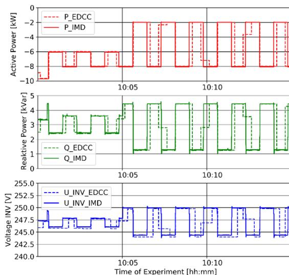
**Figure 5:** Transmitted Readings (EDCC) and independent measurements (IMD) for a time period with activated P(U) control algorithm.
