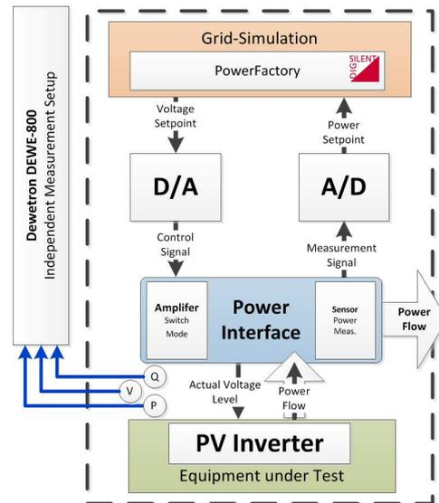
**Figure 2:** Basic principle for the PHIL part of the proposed setup describing the signal flow.
