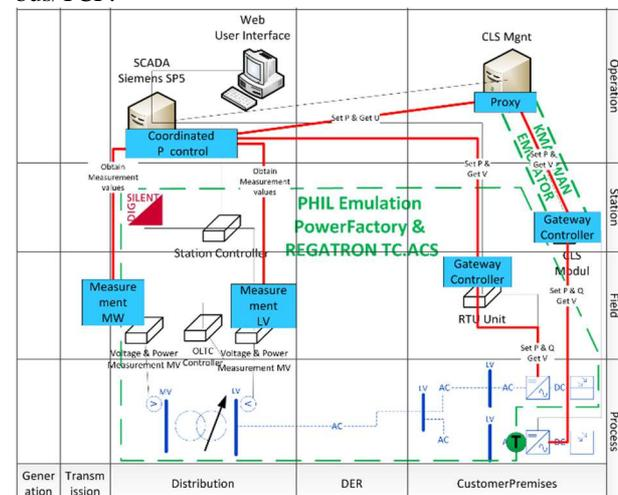
**Figure 3:** SGAM function layer diagram representing smart operation strategies for decentralized PV-Systems
