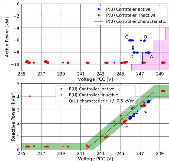
**Figure 4:** Comparison of the coordinated P(U) control governed by the EDCC and the Q(U) control of the inverter. Control characteristics are represented by the purple respectively green lines.
