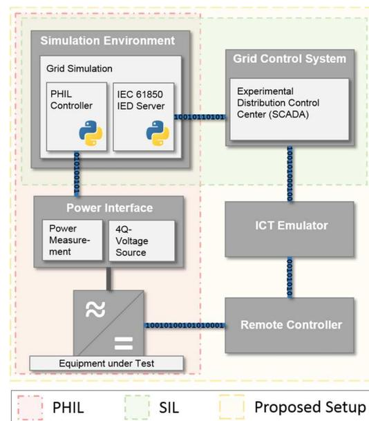
**Figure 1:** Schematic illustration of the SIL, PHIL and the proposed setup.
