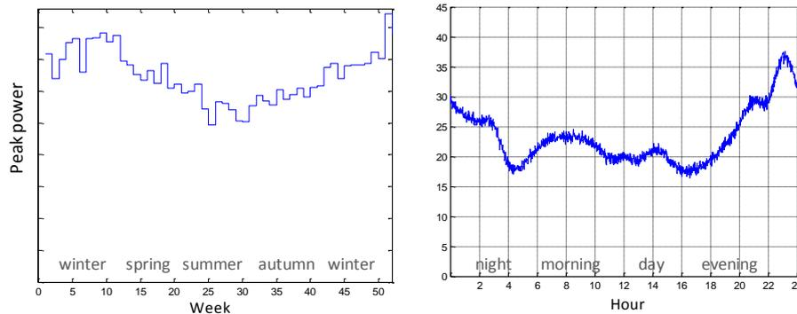
**Figure 4—35: Annual (a) and daily (b) load curves of residential customers (electric heating with a water storage)**
