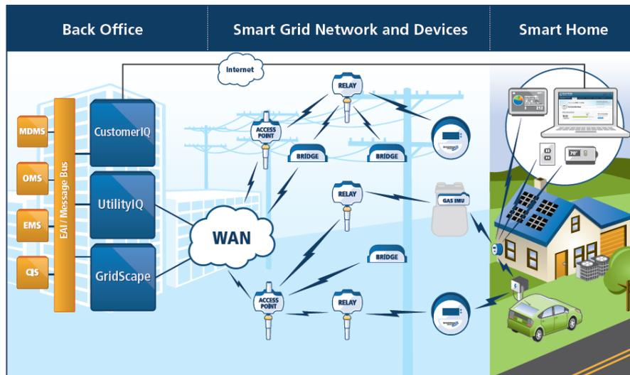
Figure 4—22: RF Mesh Smart Grid architecture
