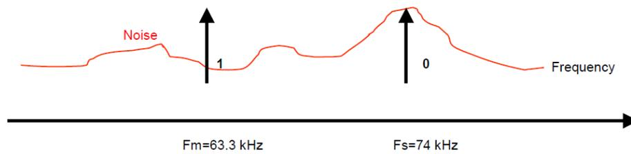
**Figure 4—18: Spread-frequency shift keying frequency spectrum**
