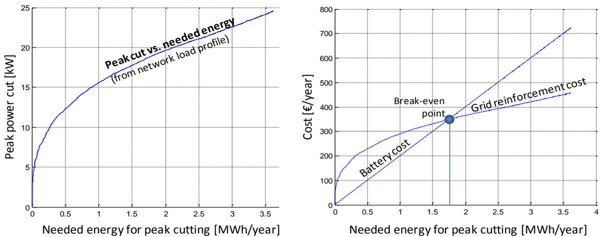
Figure 4—36: a) Peak cut vs. needed energy (taken from the network load profile) b) Economic limit for peak cut
