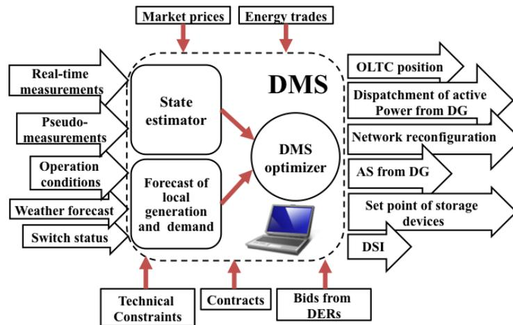
Figure 4—4 – Advanced DMS application architecture for the optimal active operation of distribution networks [21]
