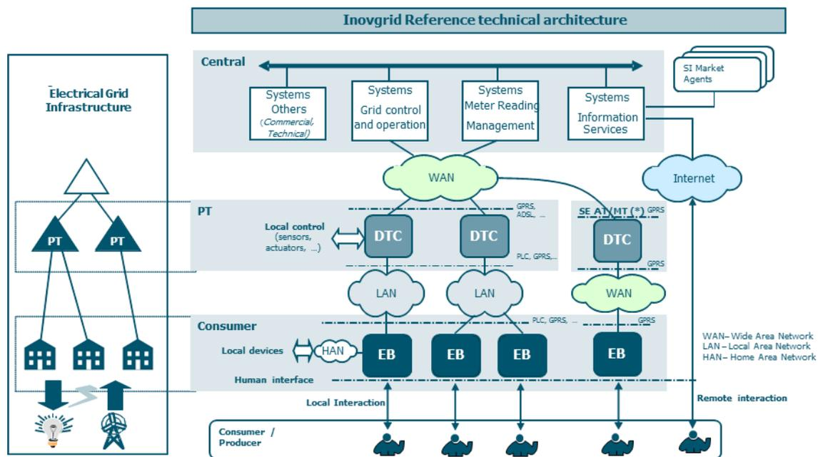
Figure 4—16: InovGrid pilot-project reference architecture
