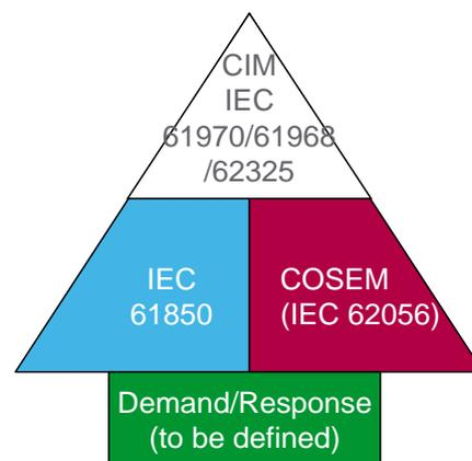
Figure 5—3: IEC main semantic domains (power supply side)
