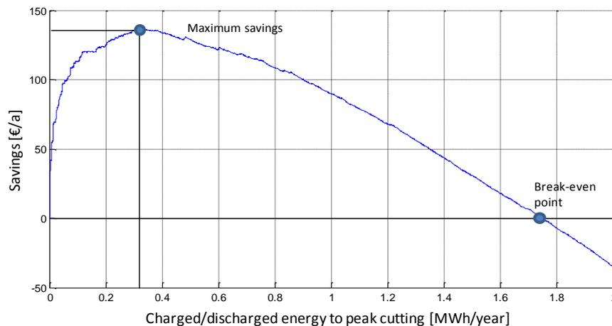
Figure 4—37: Savings vs. needed battery capacity (charging/discharging)
