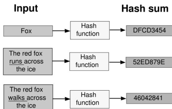
**Figure 4—25: Hash Function operation**
