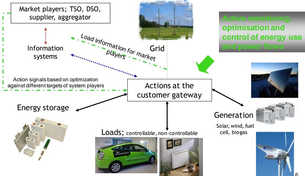
Figure 4—28: Customer grid connection (gateway) in the Smart Grid concept
