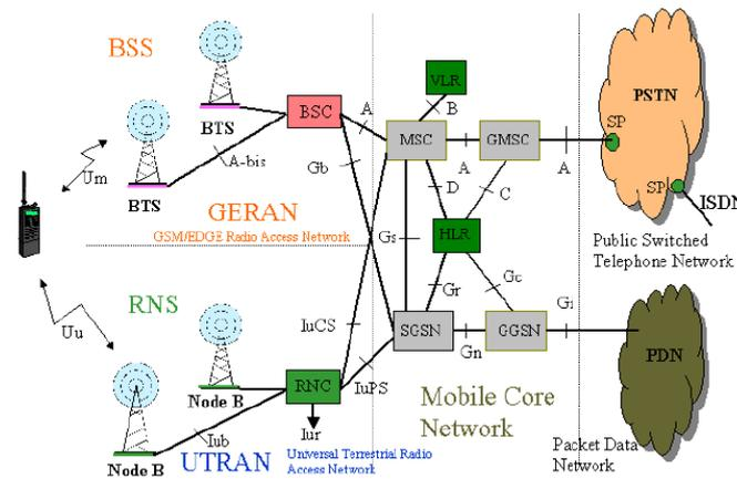
**Figure 4—23: Mobile network operator infrastructure**
