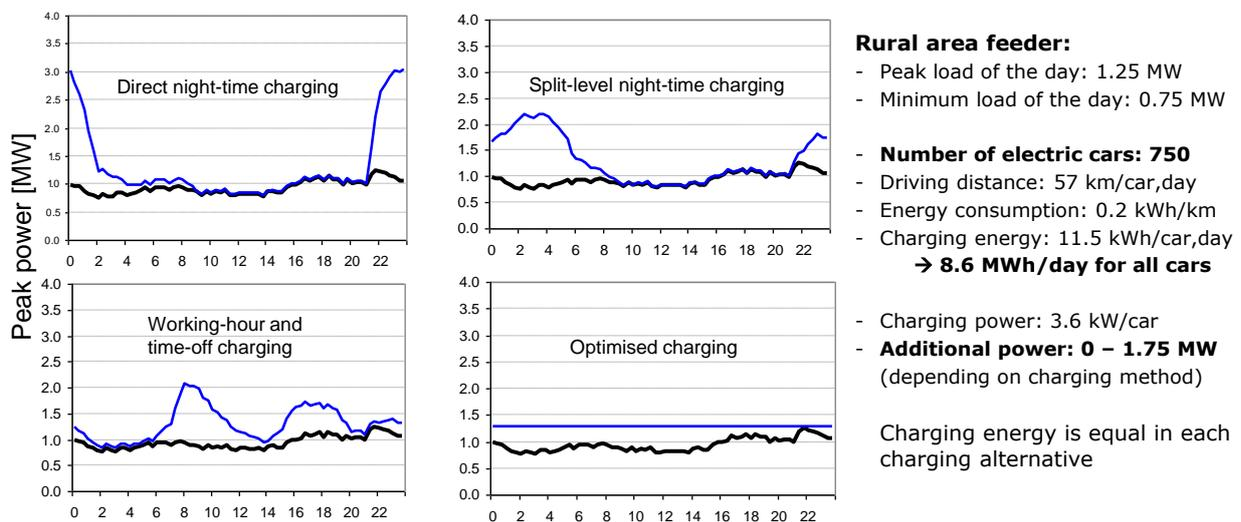
Figure 4—29: Impact of alternative EV charging principles on the peak power of a medium-voltage feeder
