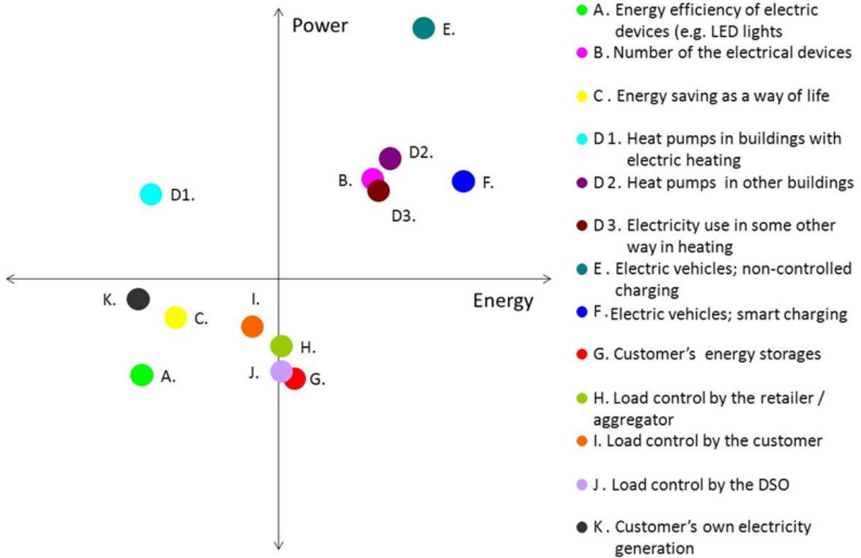
Figure 4—30: Effects of different actions on the power and energy transmitted on the distribution network
