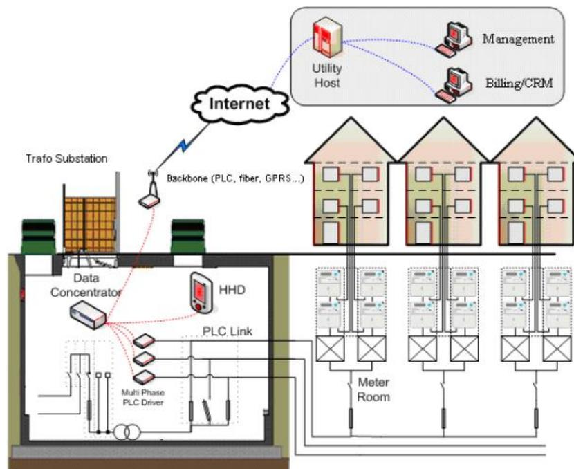
Figure 4—11: PLC Prime reference architecture
