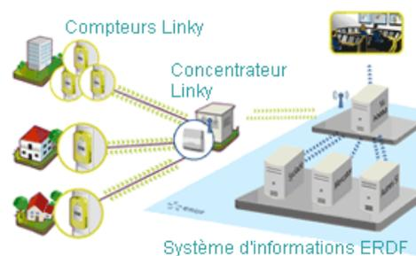
Figure 4—17: ERDF Linky system architecture
