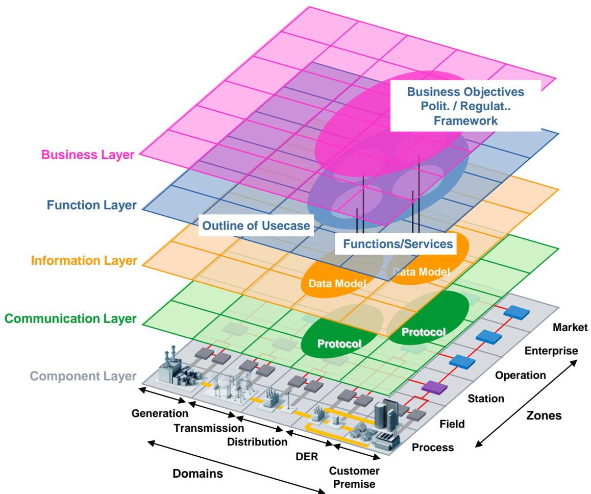
Figure 5—2: Smart Grid Architecture Model (SGAM)
