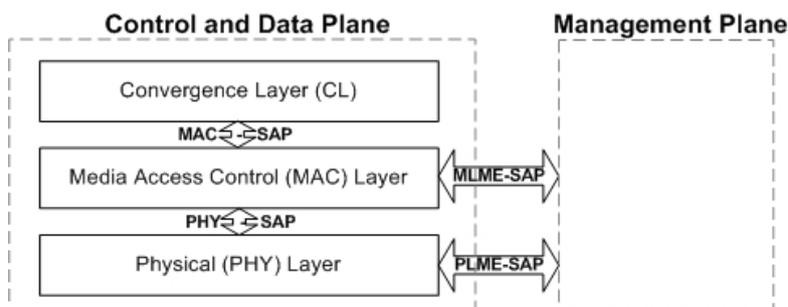
Figure 4—13: PLC PRIME lower layers protocol stack
