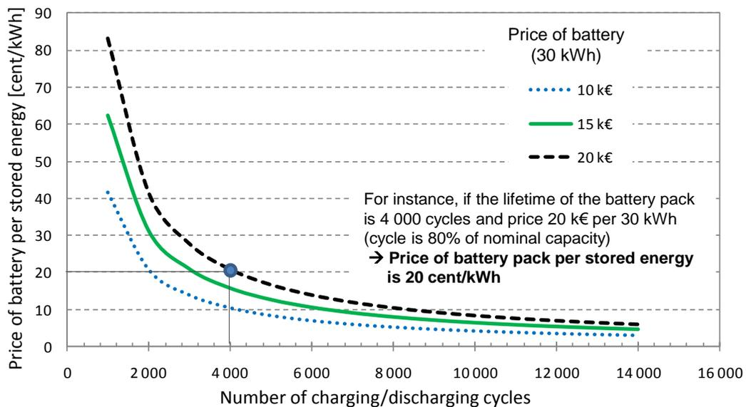
Figure 4—34: Price of battery (30kWh) per charged/discharged energy (cent/kWh) as function of their lifetime (number of charging and recharging cycles)
