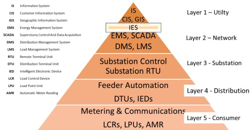
Figure 4—1: The high level architecture of a Smart Grid distribution control centre.
