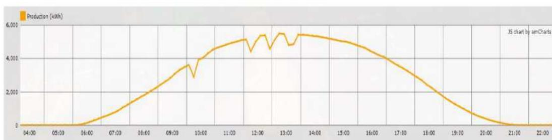
Figure 36: Example of the active PV limitation
