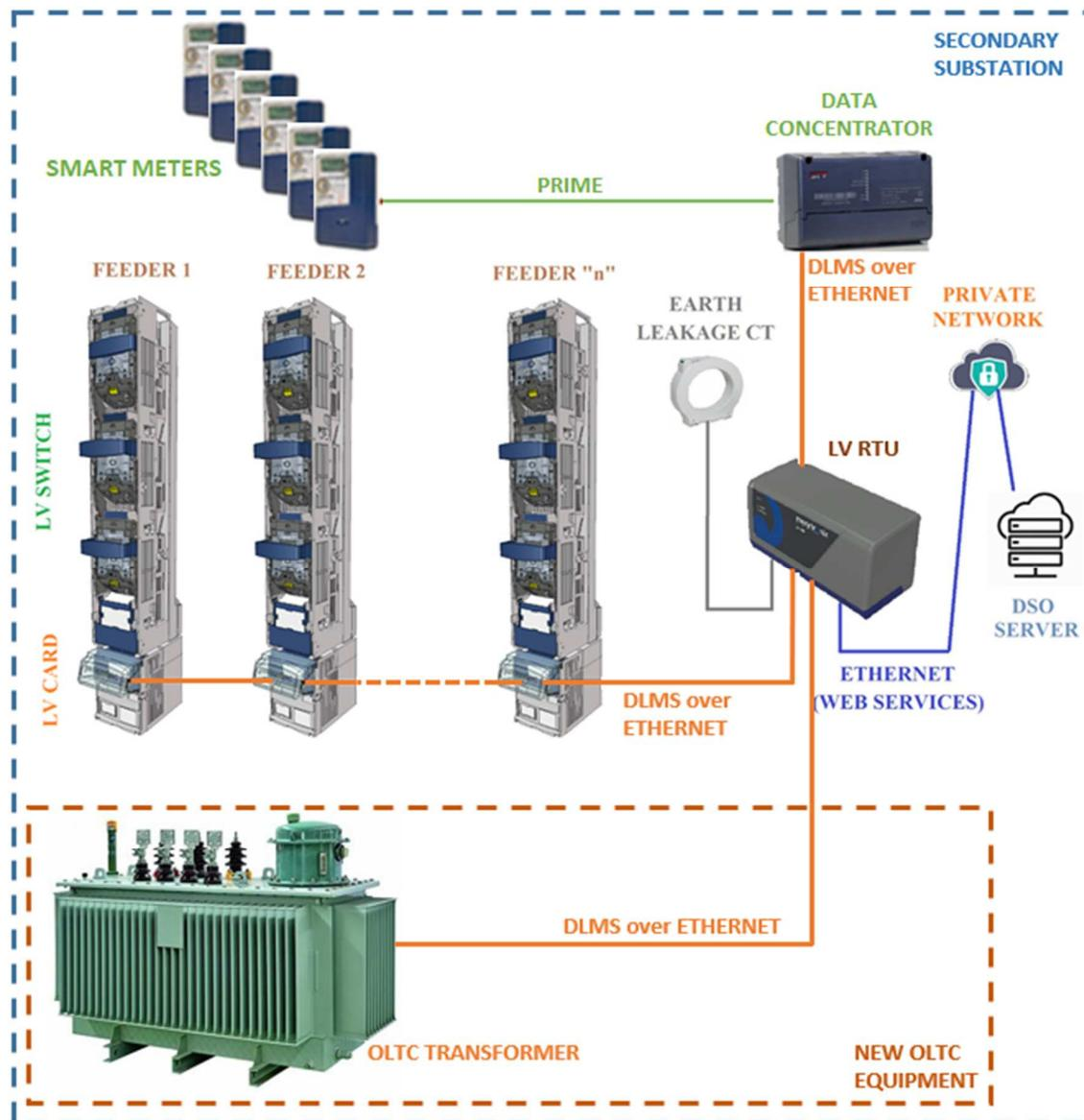
Figure 26: Use of OLTC transformers in MV/LV secondary substations<sup>10</sup>
