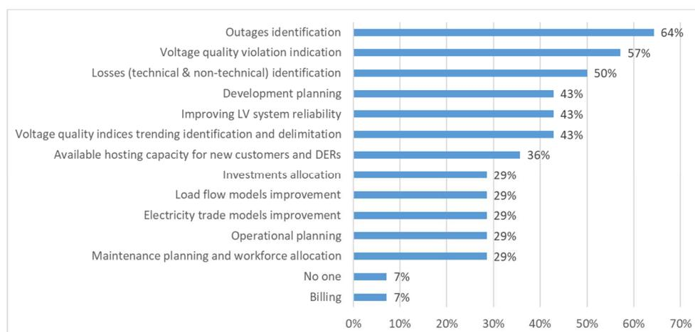
Figure 15: Use cases of the smart meters' data for LV distribution system management
