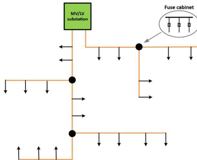
Figure 21: Example of radial network topology
