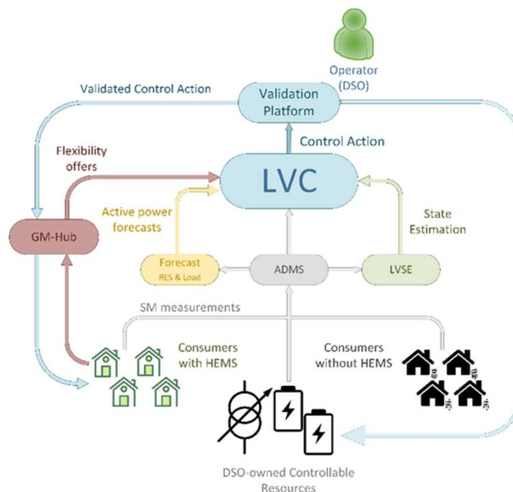
Figure 30: Proposed control for predictive voltage control in InteGrid [33]
