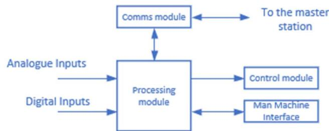
Figure 52: Smart terminal units
