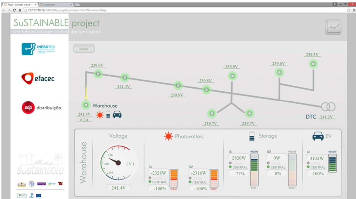
Figure 28: Synoptic of the Voltage Control Algorithm embedded in the DTC [30]
