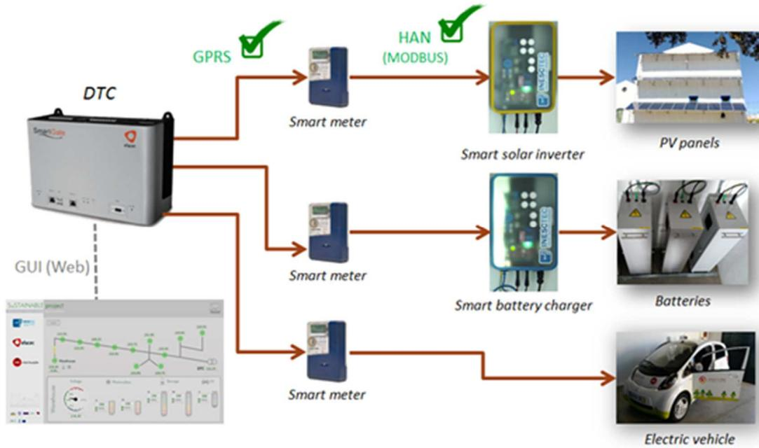
Figure 27: Voltage control demo in Portugal (communications and interfaces setup) [30]
