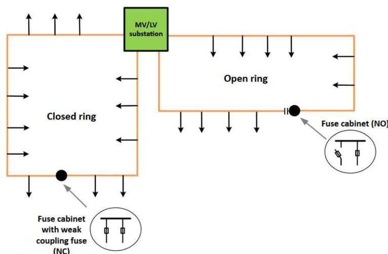
Figure 22: Example of open/closed ring network topology
