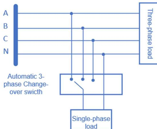
Figure 51: Automatic load-transfer switch
