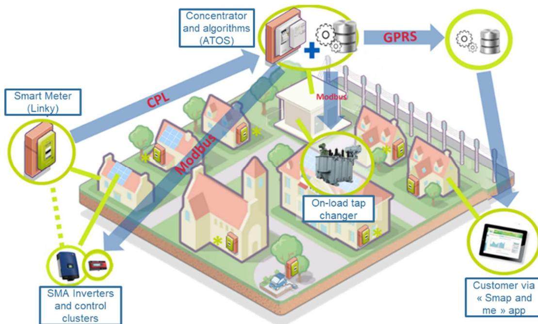
Figure 33: Architecture of the experimentation in the SMAP project
