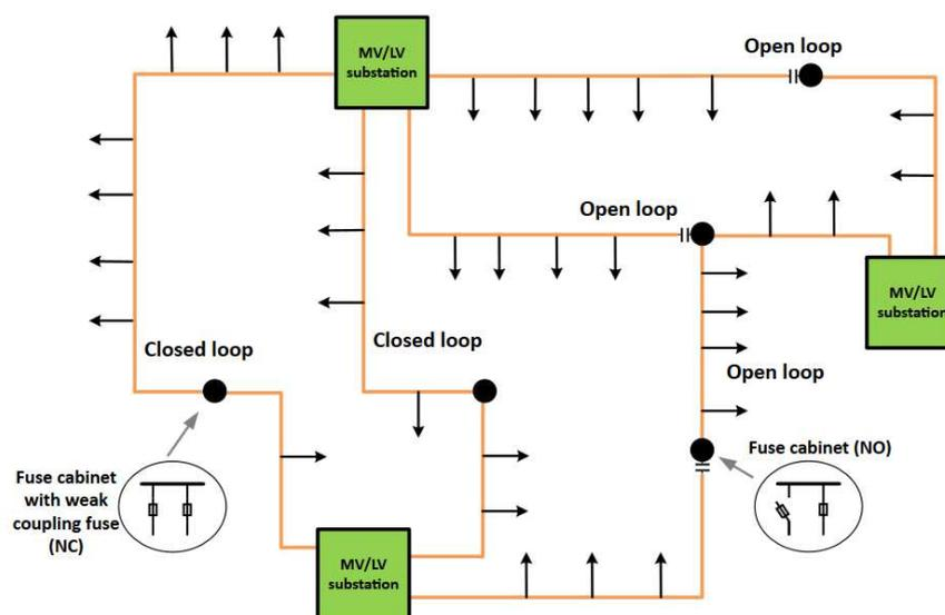
Figure 23: Example of open/closed loop network topology
