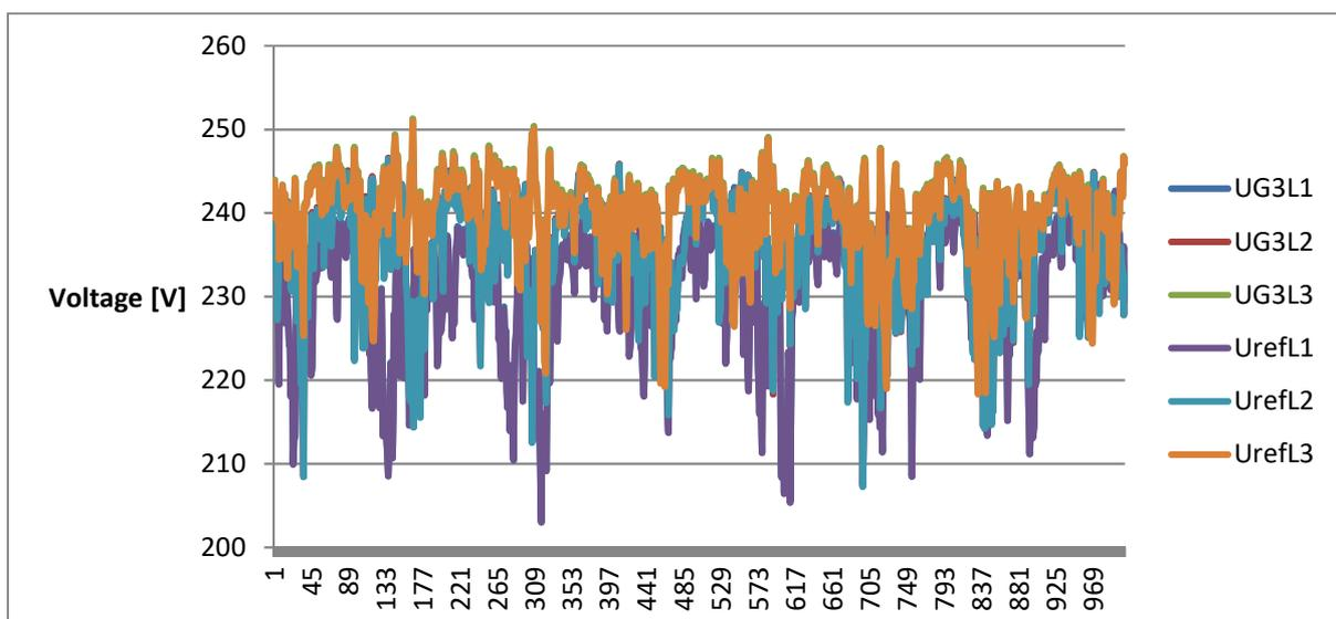
Figure 17: Voltage measurements from a PQ analyzer and a smart meter
