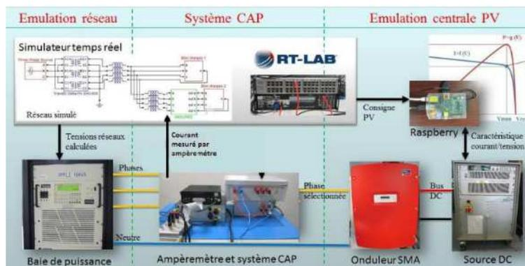
Figure 49: Real time simulation model [82]
