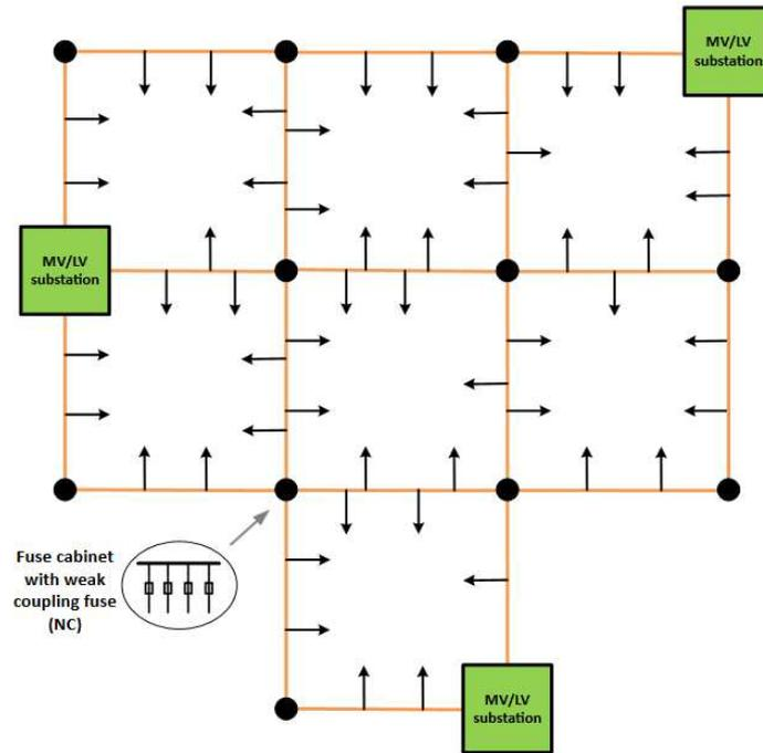
Figure 24: Example of mesh network topology
