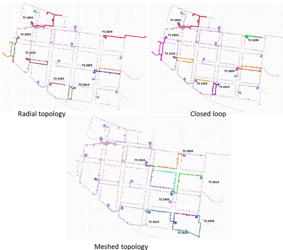
Figure 25: Radial, closed ring and simple mesh network topology
