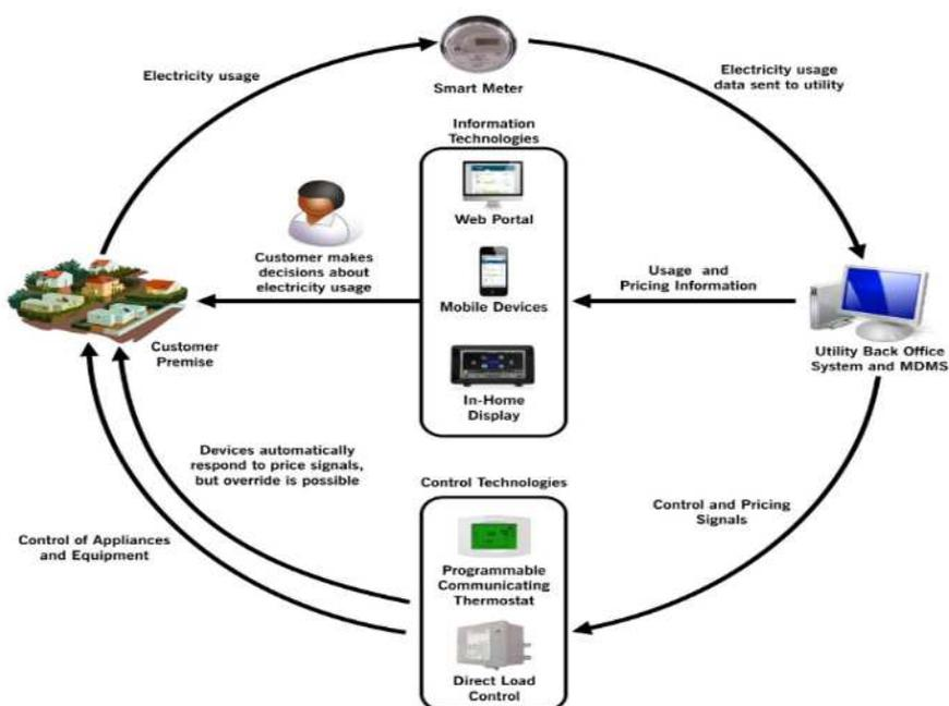
Figure 43: Advanced Measurement Structure [63]
