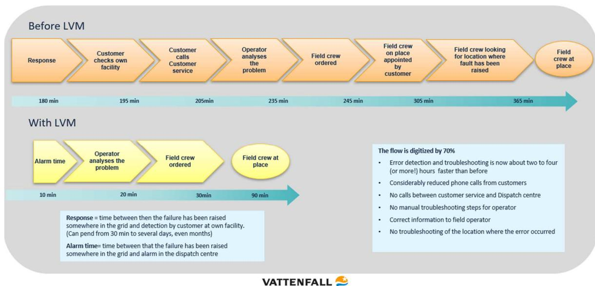
**Figure 18: Savings in time achieved by implementation of LVM – Pilot project Low Voltage Monitoring performed at Vattenfall Eldistribution -Sweden through period 1 January 2016 - 30 September 2016**
