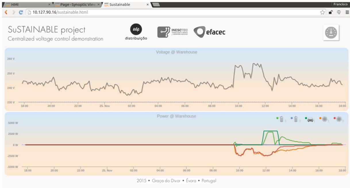
Figure 29: Detailed voltage and load profiles [30]
