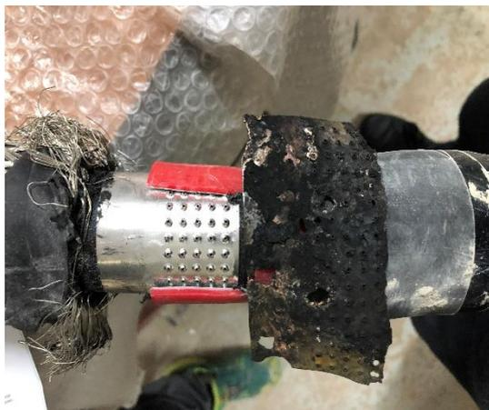
Figure 3-12: Comparison of a damaged "cheese grater" and a new grater.
