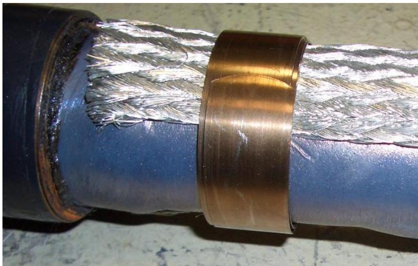
Figure 2-4: Screen connection by a copper braid and constant force spring.
