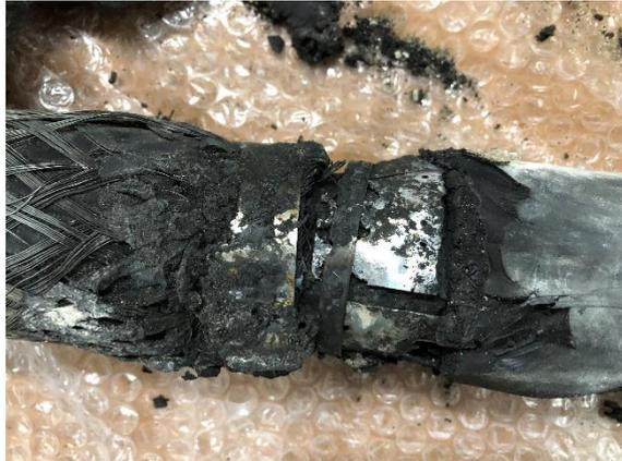
Figure 3-10: Damaged cable with ligarex.
