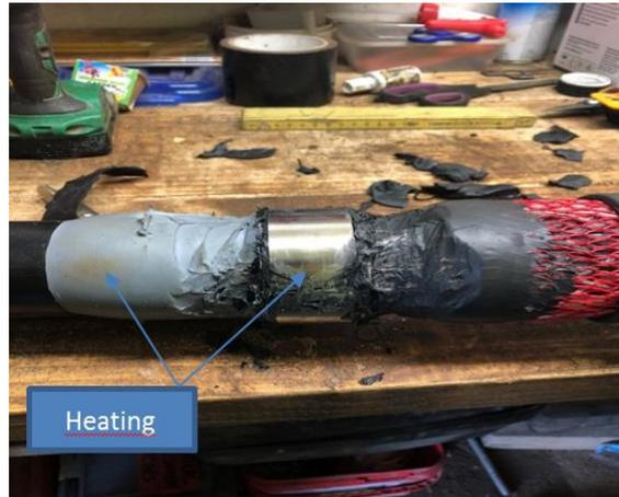
Figure 3-15: Joint opened at roll spring location.
