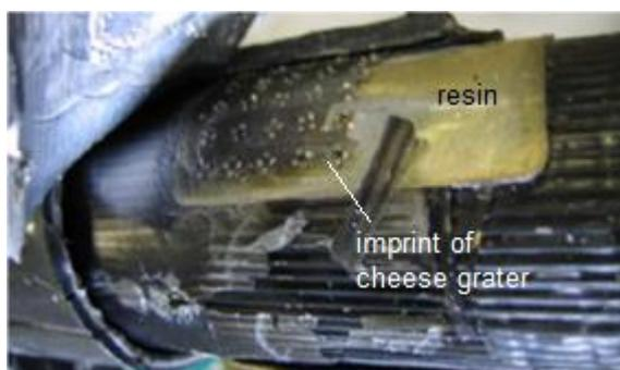
Figure 3-5: Presence of resin between "cheese grater" and Al cable screen.
