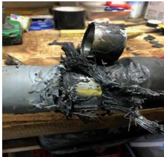
Figure 3-17: Further unwrapping of roll spring.
