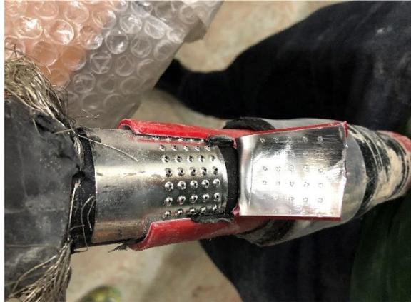
Figure 3-11: "Cheese grater" and aluminium screen and laminate.
