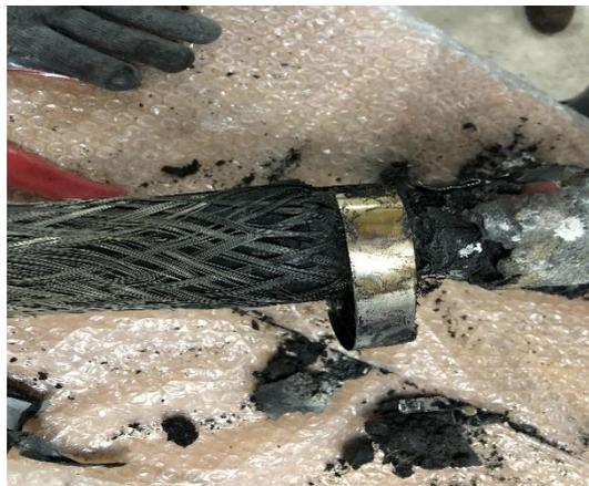
Figure 3-13: Damaged cable with ligarex and aluminium screen.
