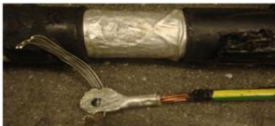
Figure 3-1: Missing laminate grounding (66 kV 150 mm<sup>2</sup> Al TSLE).
