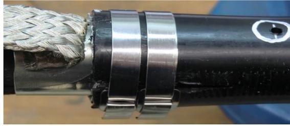
Figure 2-5: Screen connection by a screen plate and cable clamp ('Ligarex') (Main french networks solution solution).
