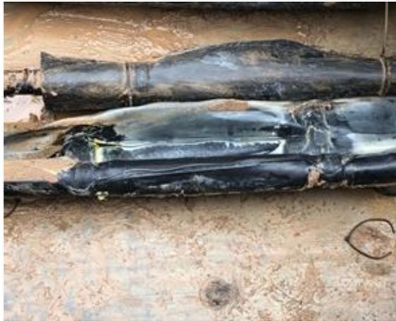
Figure 3-14: Faulty 630 mm<sup>2</sup> Al cable.
