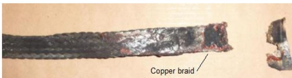
Figure 3-8: Cable outer sheath and rest of screen device ("cheese grater").
