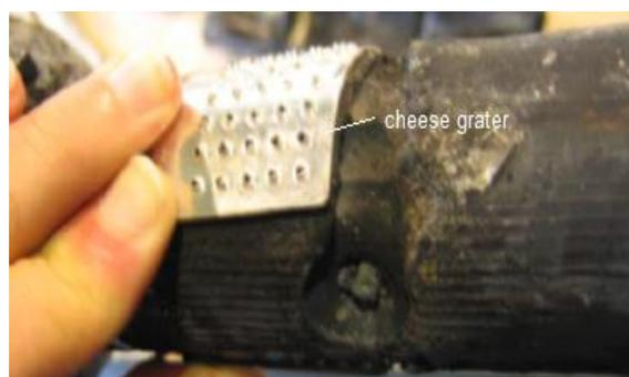
Figure 3-6: Damage of external semi-conductive layer with a new grater to show the initial position.
