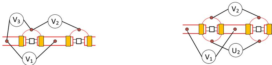
(a) Voltage measurement connection points for a cable with one screen connection device.
