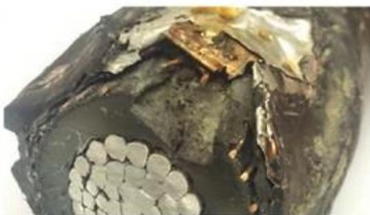
Figure 3-3: Missing laminate grounding (24 kV 400mm<sup>2</sup> Al TSLE), [11].
