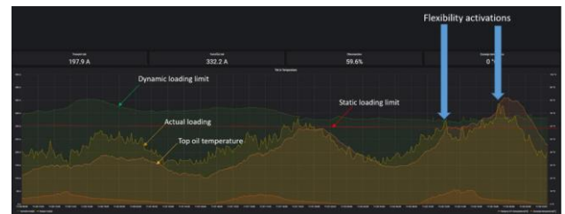
Figure 47: Multi physics thermal mode, load, oil temperature and resulting dynamic load limit at distribution transformer- Paper 10986
