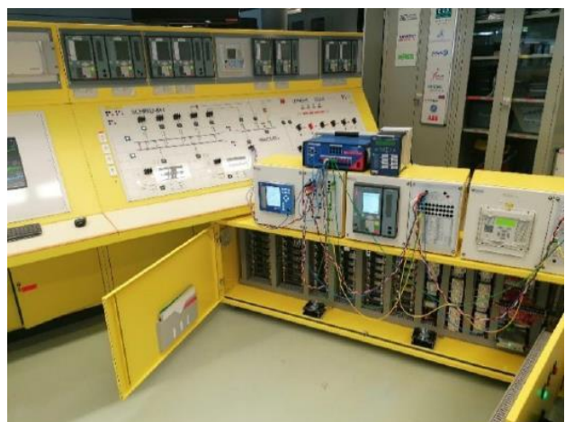
Fig. 7: Hardware model for reproducing frequency events with UFLS relays at a reduced voltage/current scale.
