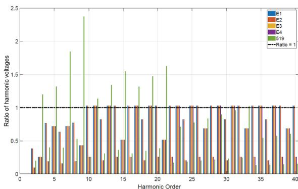
Fig. B4-3: Utilization of voltage harmonic limits for all 4 considered variants of IEC and for IEEE519 [B4-0932(US)]
