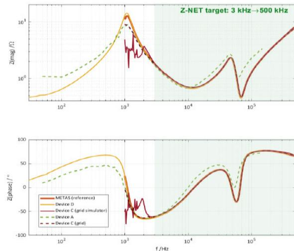
Fig. B4-4: Results of the comparative energized measurements of the Z-NET Static Impedance Reference [B4-1150(CH)]
