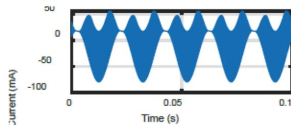
Fig. B1-5: Test residual current, half-wave pulsating, 50 Hz and supraharmonics [B1-0060(SE)]
