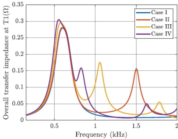
Fig. B3-3: Overall transfer impedance at wind park terminal for four cases [B3-0135(SE)]
