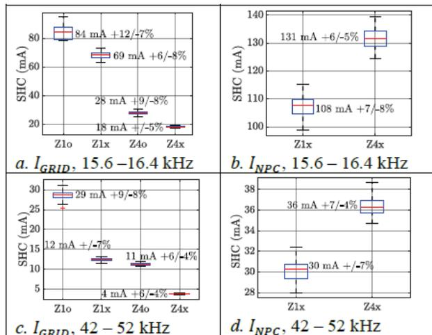
Fig. B3-6: Characterization of SH variations (x/o: neighbouring devices on/off; Z1/Z4: cable to supply transformer shortest/longest)
