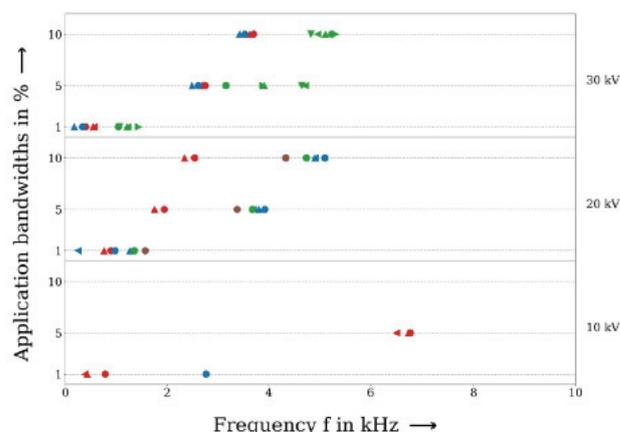
Fig. B3-12: Application bandwidth of medium voltage VTs determined with 1 MΩ SFRA [B3-0230(AT)]
