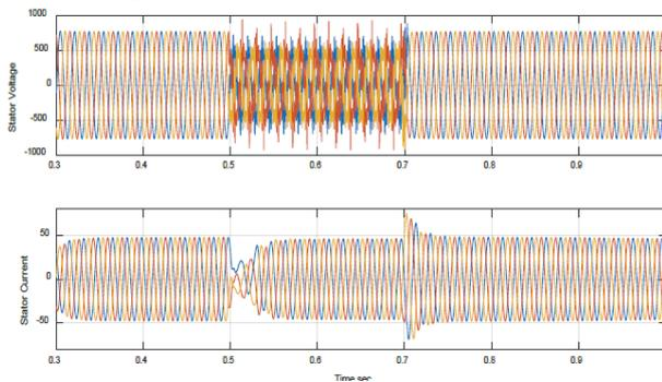
Fig. B2-9: Stator voltage and current with STATCOM and three-phase RL impedance only during faults [B2-0132(EG)]
