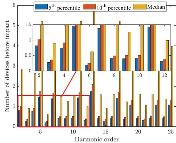
Fig. B4-6: Safe harmonic hosting capacity for 60'000 LV customers, presented in 5<sup>th</sup> percentile, 10<sup>th</sup> percentile and median [B4-0076(SE)]
