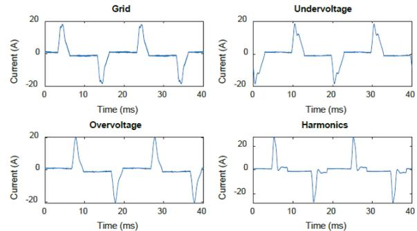
Fig. B2-8: Current waveform for four identical groups of lamps fed by different voltage profiles [B2-0077(SE)]
