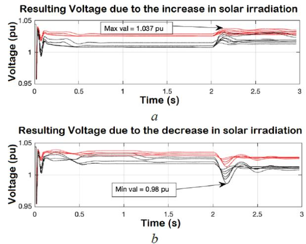
Fig. B4-16: Impact on the CCP voltages with CCP1 voltages (red) and CCP2 voltages (black) in case of an increase (a) or decrease (b) in solar irradiation [B4-0193(BR)]
