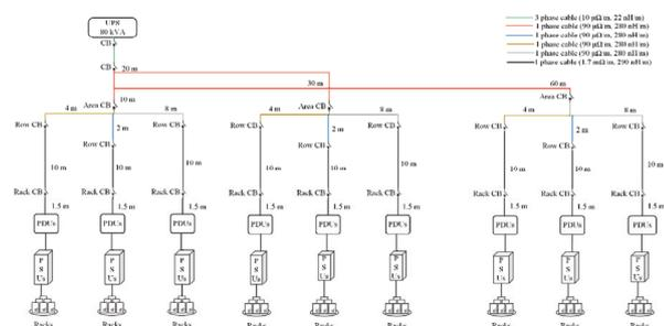
Fig. B4-15: The studied IPSS structure of the data centre [B4-0090(SE)]
