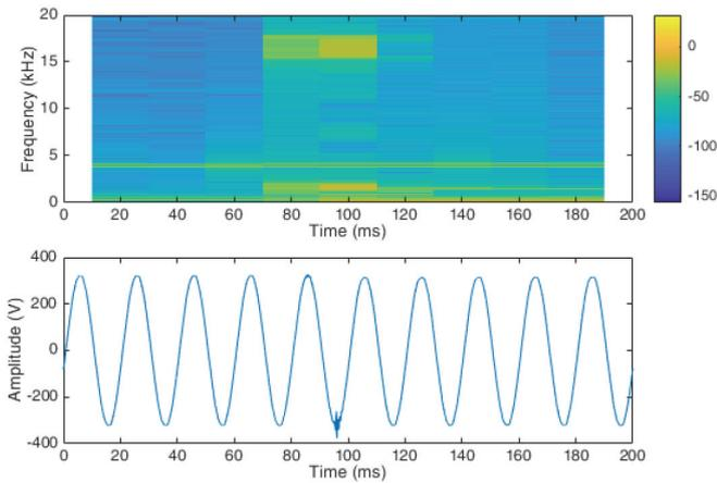
Fig. B4-5: STFT of oscillatory transients from the PV panel [B4-0049(SE)]
