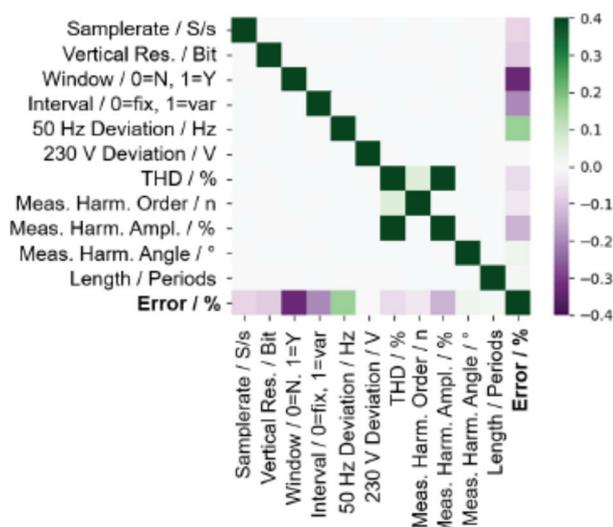
Fig. B3-11: Result of the correlation analysis for a PQI with variation of the whole state space for all parameters [B3-0945(DE)]
