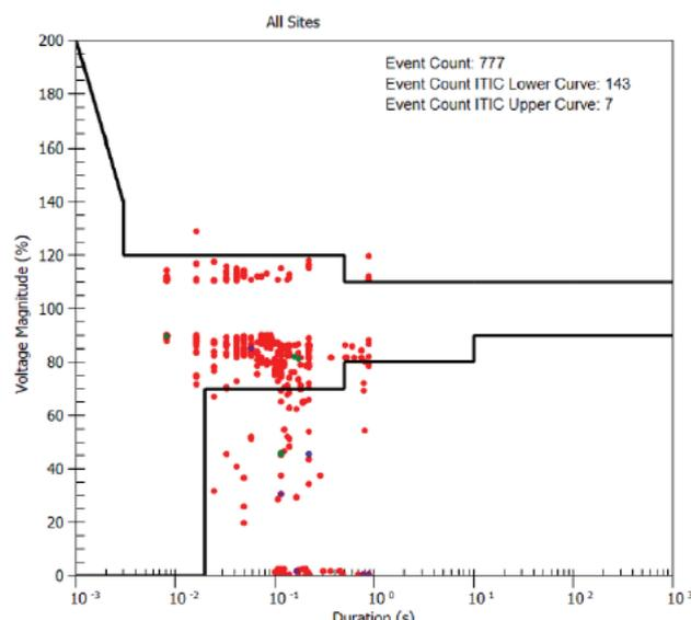
Fig. B3-9: RMS Variation Magnitude-Duration Scatter Plot Displaying Voltage Dips with Load Loss [B3-0961(US)]
