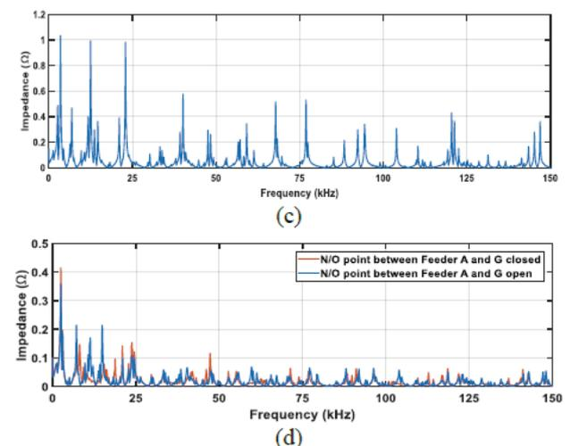
Fig. B3-7: MV Test Network Frequency Scan at Node 101 with (c): Feeder A, B, C and D and (d): Feeder A, B, C, D, E, F, G and H connected [B3-0023(SE)]
