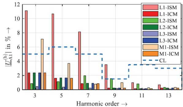
Fig. B2-10: Voltage harmonics for load scenarios measured in interconnected (ICM) and island (ISM) mode [B2-0305(GE)]
