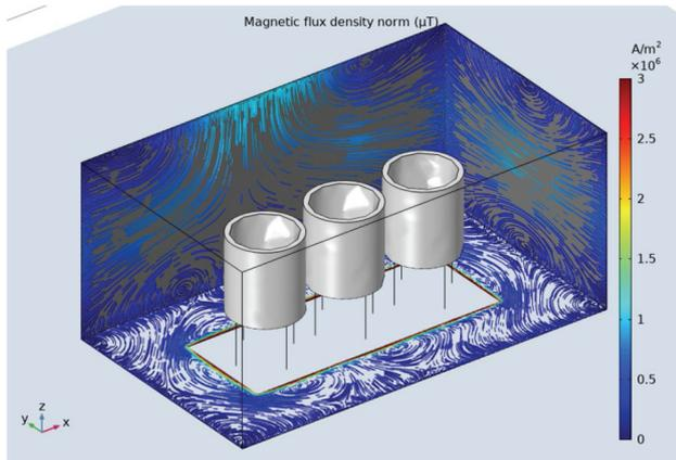
Fig. B1-1: Current density streamlines inside the inner Al shield for the solution with partly covered floor [B1-0238(IT)]
