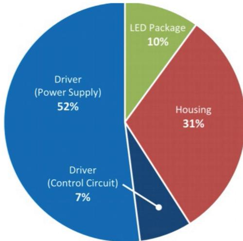
Fig. B1-6 Distribution of LED failures (Source: Appalachian Lighting Systems, Inc.) [B1-0026(SE)]
