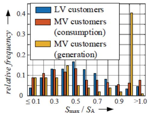
Fig. B4-1: Histogram of the ratio between maximum observed power and agreed power [B4-0065(DE)]
