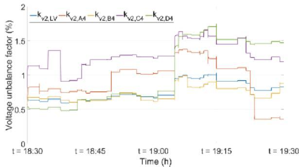
Fig. B2-3: Voltage unbalance factor without local storage [B2-0263(UK)]
