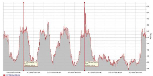
Fig. B2-4: Weekly profile of total harmonic voltage distortion at a fast charger terminal [B2-0252(NL)]
