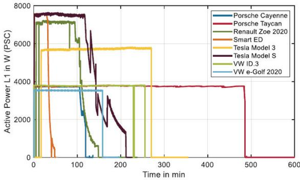
Fig. B2-5: load profiles of 2 phase and 3-phase charging EVs in active power [B2-0503(GE)]
