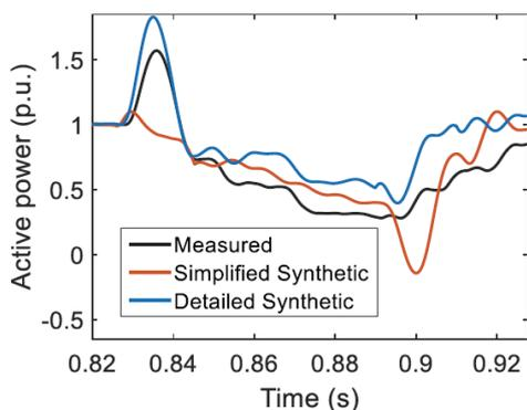
Fig. B2-2: Difference in active power between measured, simplified and detailed synthetic dip profile [B2-0184(SE)]
