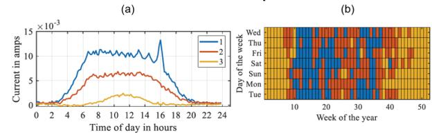
Fig. B4-10: Deep learning results for interharmonics between 50 and 100 Hz: (a) reconstructed patterns, (b) patterns spread over one year [B4-0160(SE)]
