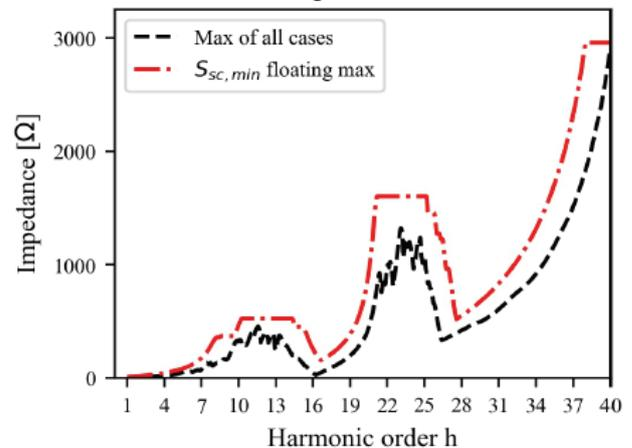
Fig. B3-2: Comparison of simplified method with the full analysis for Vores Elnet grid [B3-0440(DK)]
