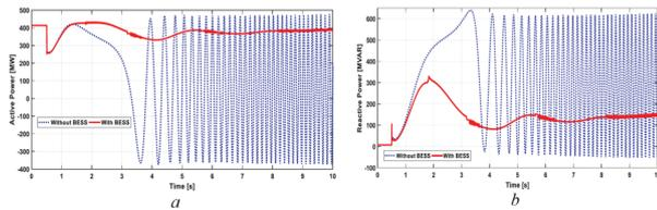
Fig. B4-14: Inter area power flows due to disconnection of interconnecting tie-line for a) active and b) reactive power [B4-0085(EG)]
