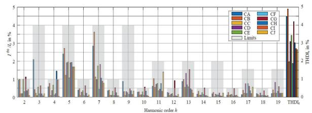
Fig. B2-7: Harmonic current emission of fast chargers in China (in % of rated current) [B2-1151(CN)]
