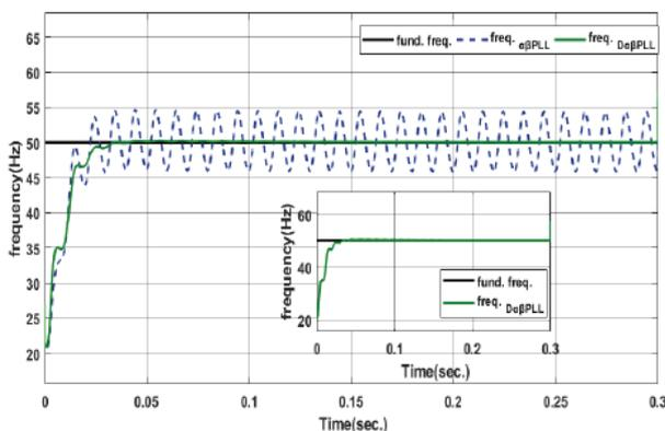
Fig. B3-10: Fundamental frequency estimation in unbalanced voltage conditions [B3-0309(EG)]
