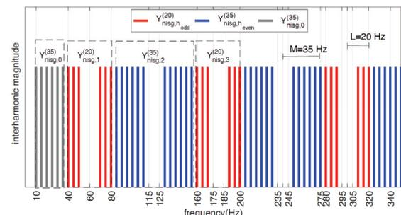
Fig. B4-2: New interharmonic subgroups corresponding to  $L=20$  Hz and  $M=35$  Hz [B4-0841(CZ)]
