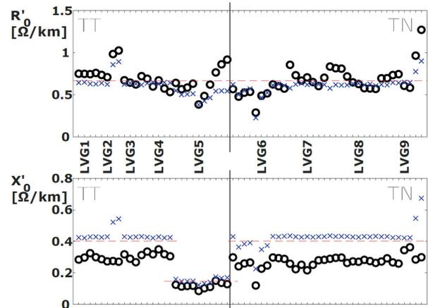
Fig. B1-3: Zero-sequence resistance (top) and reactance (bottom) per unit length of all cable sections evaluated, (left) TT network measurements, (right) TN network measurements, red (dashed) line indicating typical cable parameters, blue crosses as calculated values with respect to earth current depth [B1-0884(DE)]
