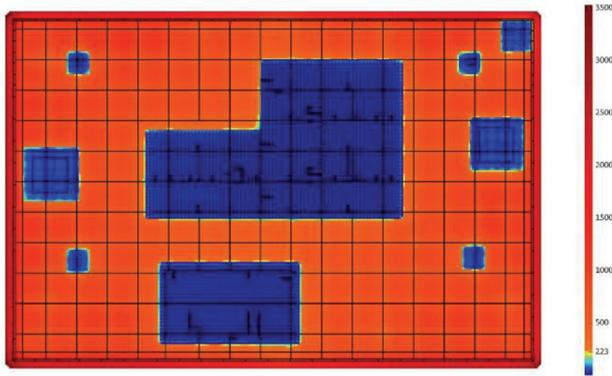
Fig. B1-4: Touch voltages results for the novel earthing grid design solution – red: unsafe areas, except for the insulated fence, blue: safe with steel mesh reinforced pavement [B1-0838(PT)]
