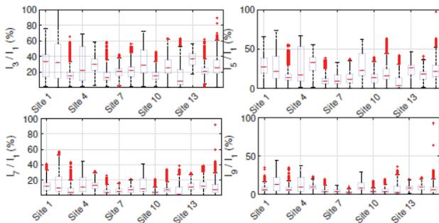
Fig. B3-1: Boxplot for harmonic current magnitudes at different measured sites [B3-0351(SP)]
