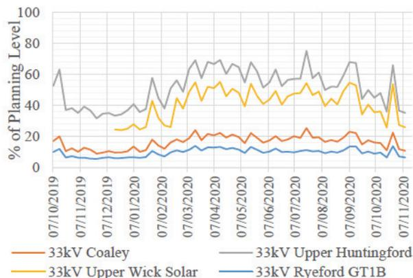
Fig. B4-8: Weekly 95<sup>th</sup> percentile aggregates of the 16<sup>th</sup> voltage harmonic at four sites with high LCT penetration [B4-0370(GB)]
