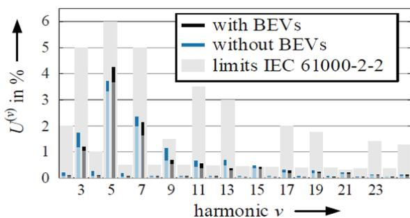
Fig. B2-6: Harmonic voltage magnitudes (95 % quantile and maximum) for long-term measurement with and without BEVs [B2-0835(GE)]
