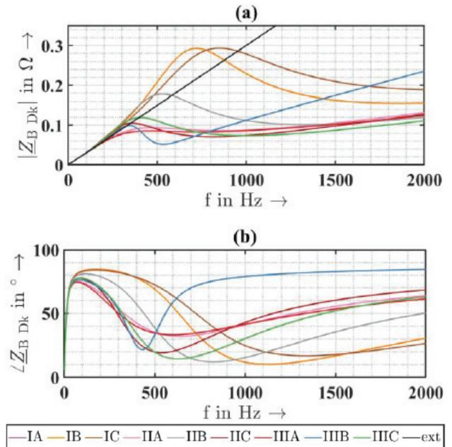
Fig. B3-4: Impedance characteristics of a urban LV network at LV busbar (a): Magnitude, (b): Phase angle [B3-0462(DE)]
