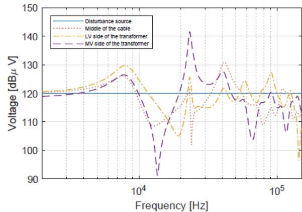
Fig. B3-5: Propagation on phase A of a 120 dBµV single-phase disturbance [B3-0101(BE)]
