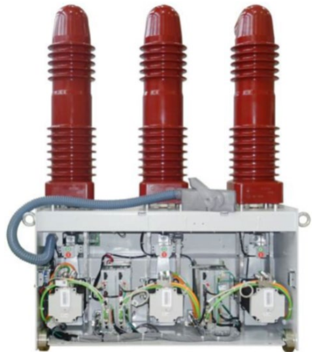
Fig. 3 from paper 0883: VD4-AF System Architecture - the operating mechanism consists of a shaft operated by a digital-controlled AC servomotor drive directly coupled with the pole structure.
