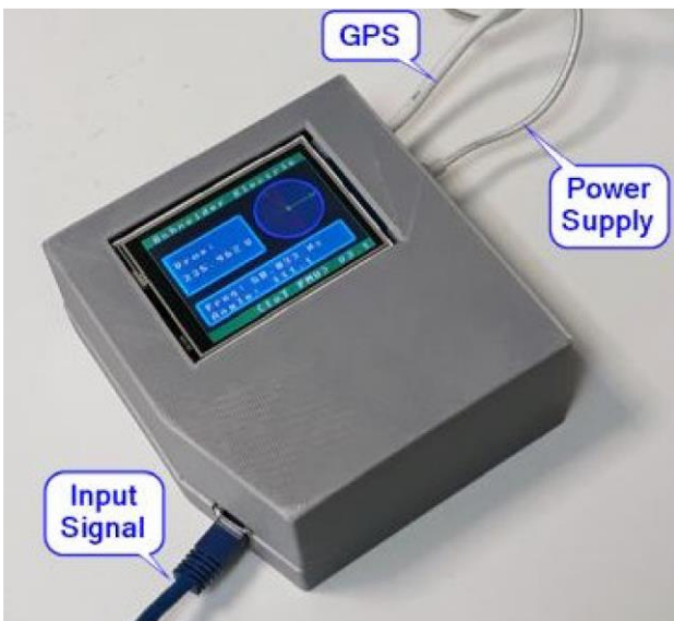
Fig. 18: PMU prototype (paper 998)
