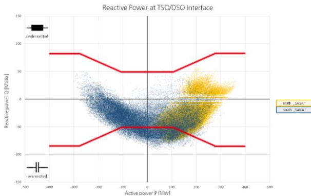
Fig. 13: Shape of reactive power exchange limits (paper 1871)
