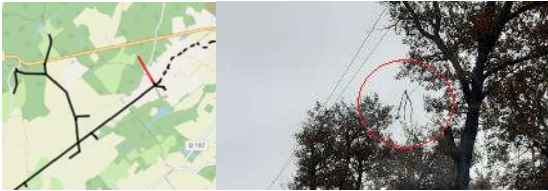
Figure 15 – LEFT: in red, the network section is likely to contain an anomaly. RIGHT: branch on the line found by field operator (©Enedis)
